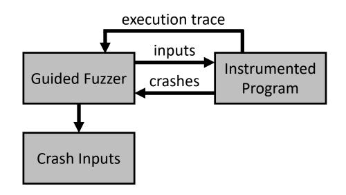
Heuristics guide genetic algorithm to generate program inputs that push the fuzzer deeper into the program control flow, avoiding the common pitfalls of fuzzers to only test "shallow" code regions.
